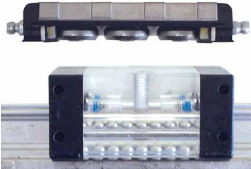
The end caps on Rollon's Compact Rail (top) are cosmetic and, even if broken in a crash, will not interfere with the operation of the slider. End caps on recirculating ball linear bearings (bottom) house the crucial rolling elements and are a potential point of failure if shattered in a crash.
