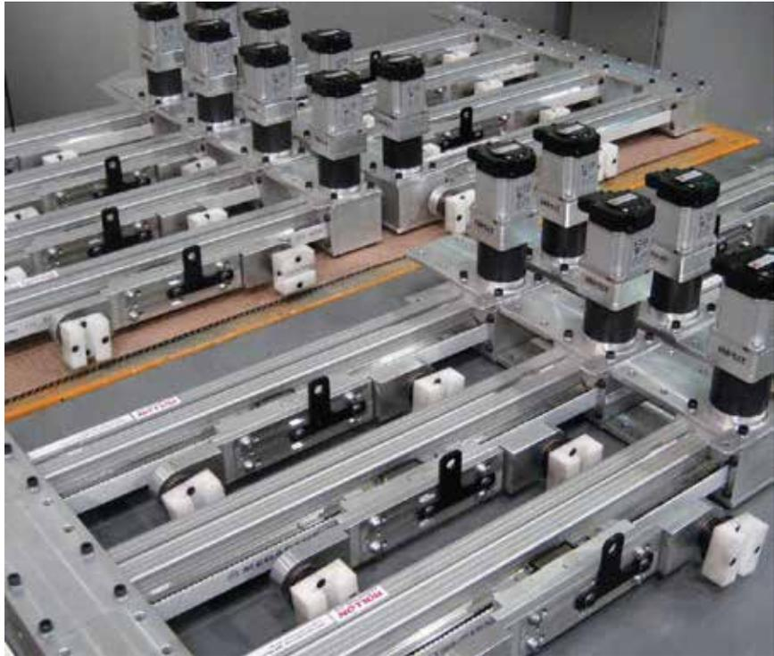
**Pactiv redesigned and replaced its original pneumatic system with a servo-driven system using Rollon's E-Smart 50 actuators. The updated system lets engineers control the timing and speed of the diversion.**
