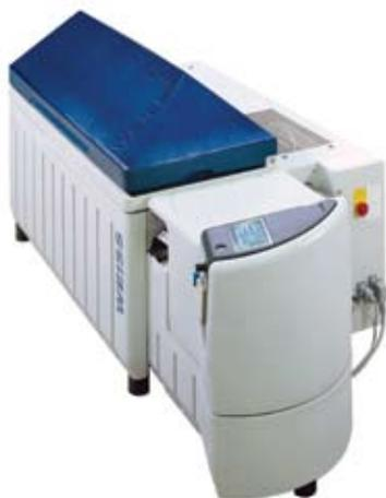
Chamber where salt spray testing was conducted in accordance with ISO 9227.
