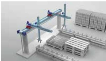
**Fig. 2 :** In certain end-of-line packaging scenarios, it makes sense to build a three-axis gantry system out of heavy-duty rigid actuators to handle heavy loads rather than using a SCARA robot with a more limited payload capacity.
