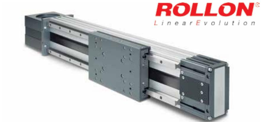
**Fig. 1** : ROBOT series belt-driven actuators from Rollon are constructed to withstand the rigors of heavy-duty packaging applications. Actuators offer speeds to 5 m/s, maximum dynamic axial load capacities from 780 to 5,510 N and stroke lengths from 100 mm to 6 m.
