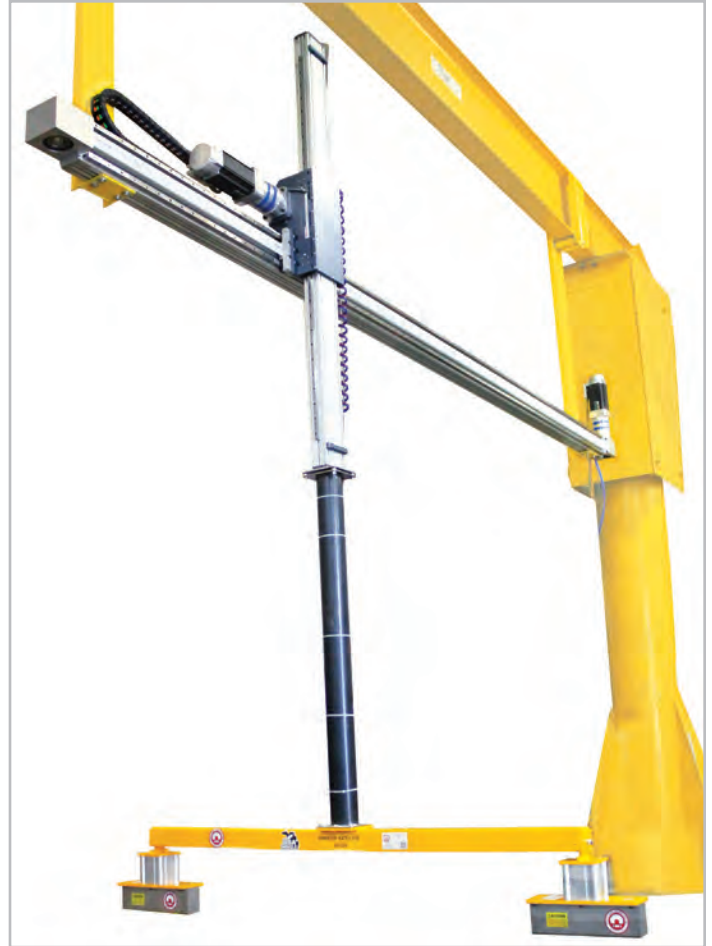
With the help of Rollon actuators, Chicago Electric designed a pick-and-place system that reduces cycle times and improves safety.
