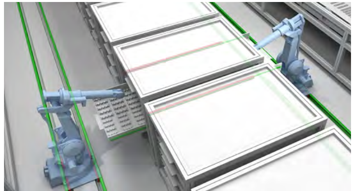
Pick-and-place robot moves along a Compact Rail axis to reach shelves positioned along the automated warehouse corridors.
