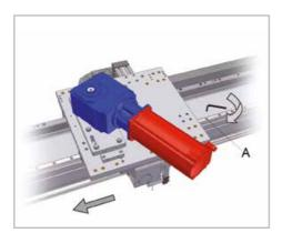
Guide (C) has a housing in tolerance, so its adjustment is much simpler. Simply put it in position and tighten the screws, with the same procedure used for the guide (G).
