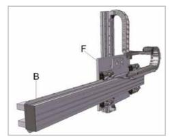
To replace a prismatic guide (B), ensure that the bearings which slide over them are discharged: for this reason, in the case of a guide on the horizontal axis, it is necessary to support the main plate or the carriage (F), so that its weight and all the equipment mounted on board, doesn't rest on bearings.
