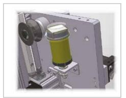
Rack lubrication is provided by an automatic greasing system (optional), which can be operated by an on/off switch located in the rear part of the lubrication unit: this unit comprises a replaceable cartridge, a pinion made form Vulkollan and adjustable lubrication frequency, depending on the particular dynamic requirements.
