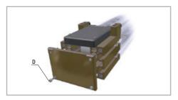
a. Remove the cover from the side opposite to the start up unscrewing the screws"D".
