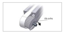
d. Remove the idle pulley extracting it laterally.
