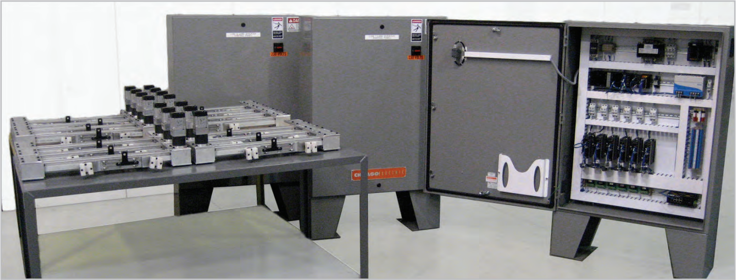
Designed and built by Chicago Electric, Pactiv's new 27-axis servo system organizes traffic flow at the end of production and resists jamming and downtime.
